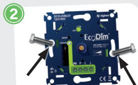
Now install the dimmer in the flush-mounting box using the screws.
