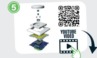
Replace the cover frame, central plate and dimmer button on the dimmer.
